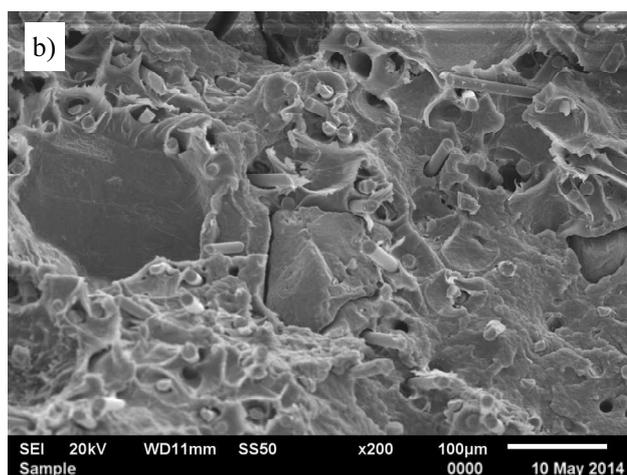
Fig. 5. Fracture microstructure: a) specimen No. 4 (PA6 + 7.5% PK + 7.5% WS), b) specimen No. 5 (PA6 + 15% PK + 15% WS); magnitude 200x
