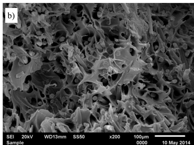
Fig. 4. Fracture microstructure: a) specimen No. 2 (PA6 + 15% WS), b) specimen No. 3 (PA6 + 30% WS); magnitude 200x
