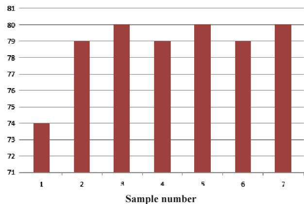
Fig. 2. Hardness measured by means of Shore method (D scale)
