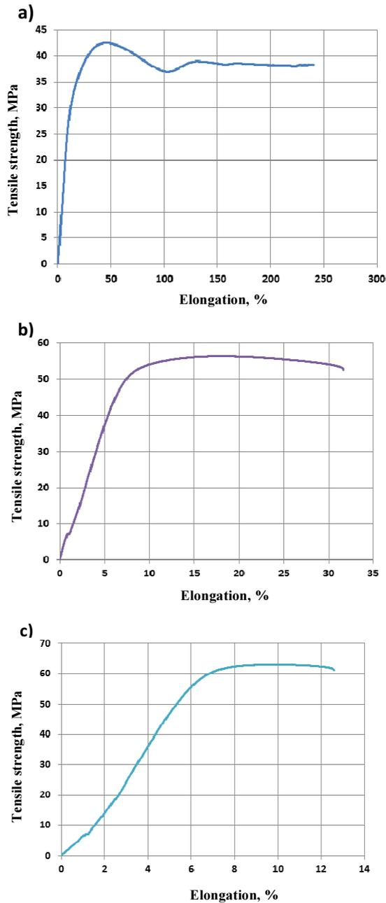
Fig. 1. Tensile strength diagrams: a) PA, b) PA6 + 7.5% PK + 7.5% WS, (c) PA6 + 15% PK + 15% WS
